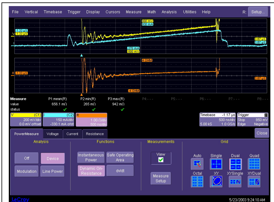
Figure 3-Measurement of the dynamic on-resistance of a MOSFET switch.
