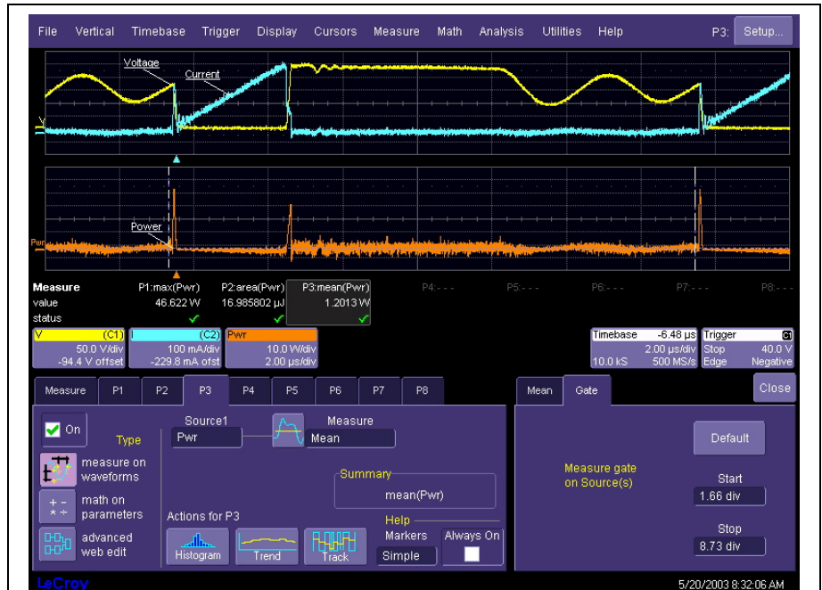
Figure 2 Measuring the average power loss per cycle
